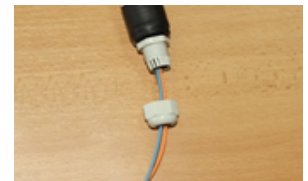
Connectors are inserted into tube through gland
